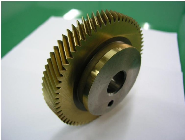
Figure N°4- Cylindrical and helical master gears coated with TiN
